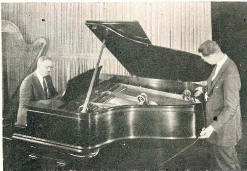
WGY'S PICK-UP DEVICE ON PIANO
